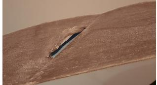
**The problem** - Not all belt joints are the same. The weakest is the taped butt joint, as above. But joins can be welded, taped, glued, and jointed in several ways. Some use the very good Norlok finger join. However most common is still the taped butt joint, as it's the cheapest to produce and it allows for the belt to be run in both directions.
